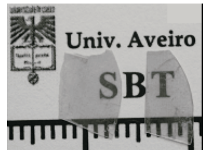
Figure 1. SBT crystals grown by the modified flux method.
