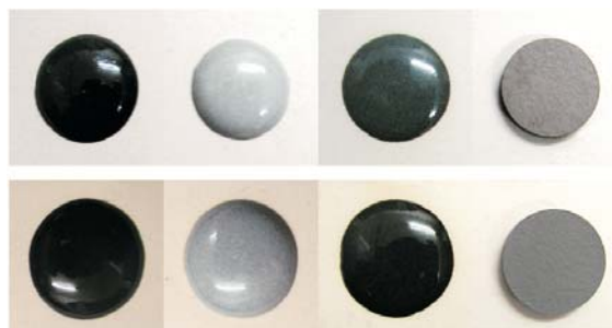
Figure 3. Examples of grey and black Co-free pigments fully based on industrial sludges (prepared in Aveiro).
