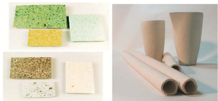
Figure 2. Examples of technical ceramics made from industrial wastes: glass-ceramics (left) and refractories based on Al-anodizing sludge (prepared in Aveiro).
